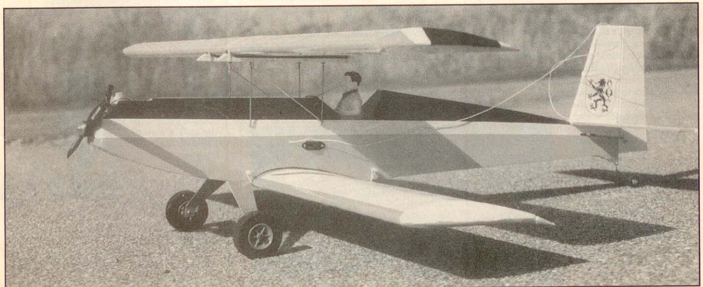
Model is very easy to take off and land. Cabane struts are ultra easy to get right, makes a change from most biplanes.
