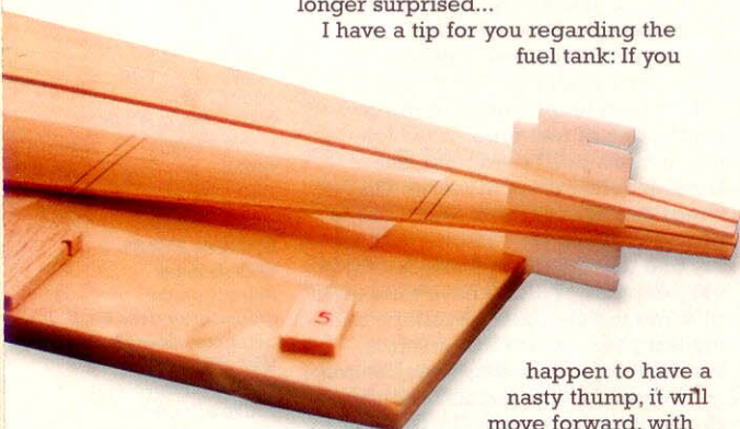
Tissan Haifa supply a handy jig which has several uses, including squaring up the rear end (as shown here).
