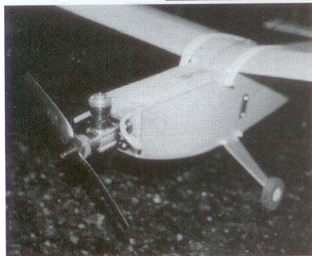
The 0.8cc engine simply bolts to the front bulkhead.
